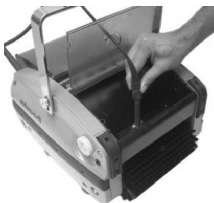
Lead the bowdencontrol under the handle into the cleanwater tray and screw together the water valve tube and the plastic nut. Be careful not to twist the bowdencontrol and test the ease of operation by pushing the red button at the top end of the stick handle.
